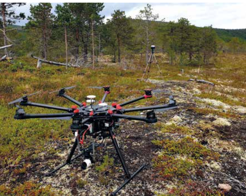
Drone borne geophysics at Tysfjord test site, Northern Norway
